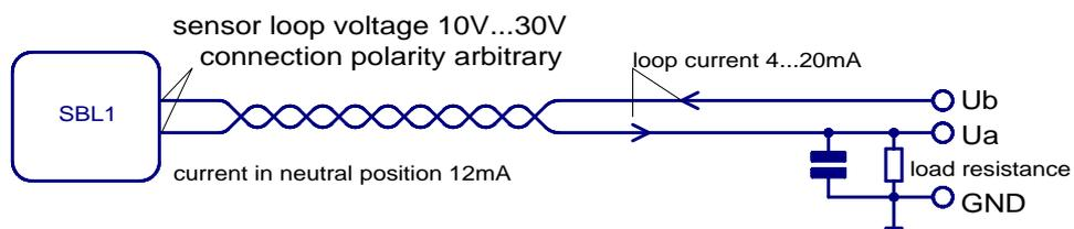
minimum loop current: 2,5mA ...3,5mA      maximum loop current: 22mA ... 26mA
